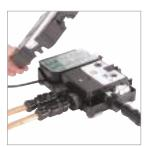
A further data cable socket has been provided for use with multiple DWM. This can be accessed by carefully snapping and removing the entry pillar and connecting the cable as described above.
