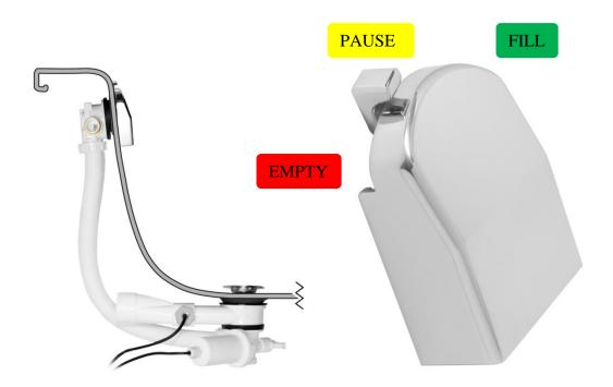
The operation could not be simpler it works like MP3 or DVD player with three states, empty, pause and fill. When the lever is in extreme left position the bath plug is open and any water drains. Turn the plug to extreme right position and the bath fills to a preset depth and temperature. At any time during filling or emptying the bath you can
