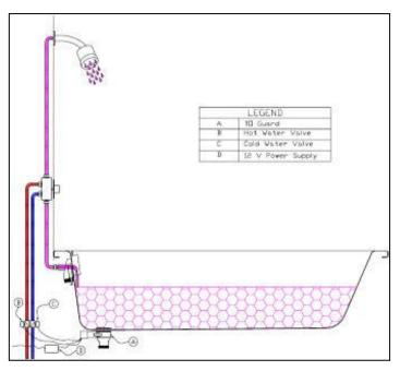
Every year in the UK around 20 people die and 570 suffer serious scald injuries due to hot bath water\*. Bathomatic TO Guard uses two sensors within the waste to gauge water temperature and weight. By constantly monitoring the bathtub water depth and temperature, the system can prevent over-hot water and overflow on any bathtub; hot and cold services will simply be closed off should they go out of pre-set, allowed ranges.
